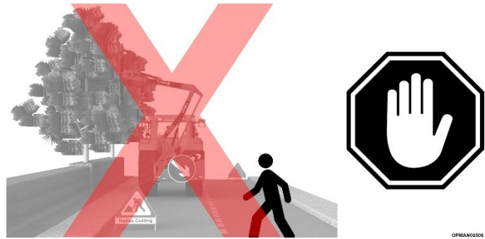
Figure 4.10 –Bystanders Out Of Working Area
