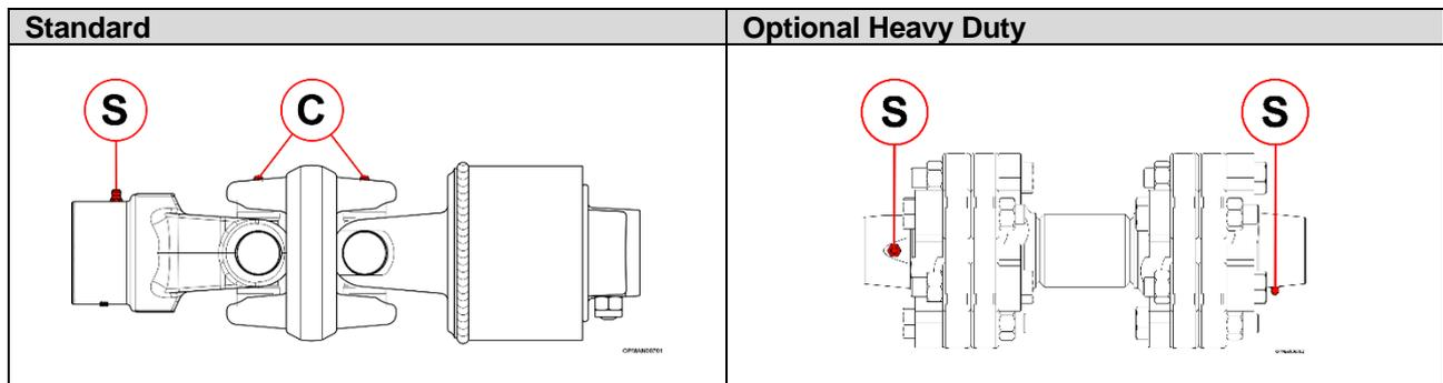
**Figure 5.6 – Multicut Connecting Shaft Grease Locations – Standard & Optional**
