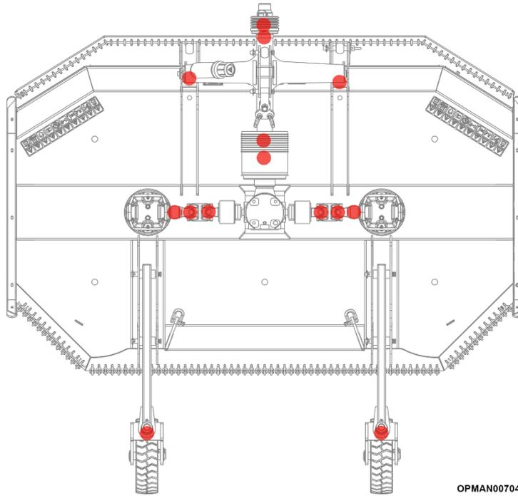
**Figure 5.7 – Multicut Grease Point Locations**
