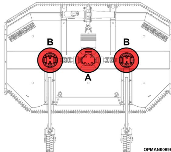
**Figure 5.1 - Multicut Gearbox Oil Capacity Locations**
