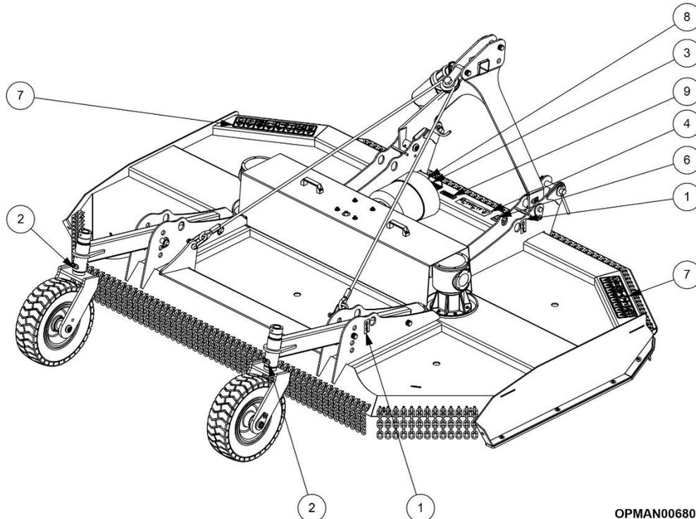
**Figure 2.3 – Multicut 300 Safety & Instructional Decal Placement**
