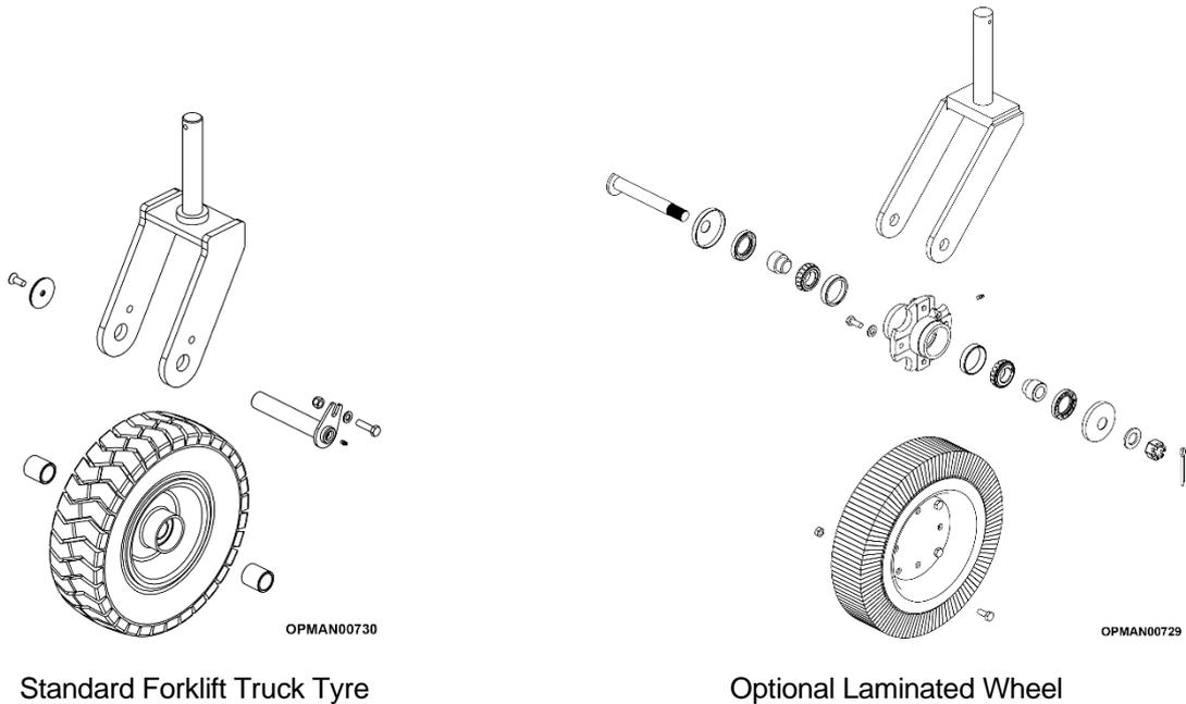
**Figure 5.33 – Multicut Wheel & Fork Assembly**
