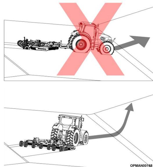
Figure 4.21 – Approach Ditches At An Angle
