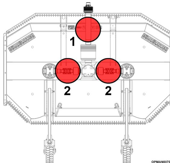
**Figure 5.4 – Multicut Input Shaft Type Locations**
