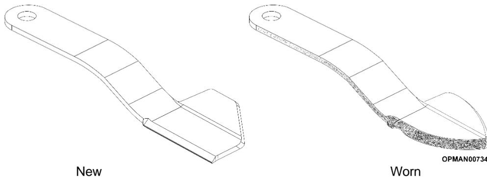
**Figure 5.18 - Standard Multicut Blades**
