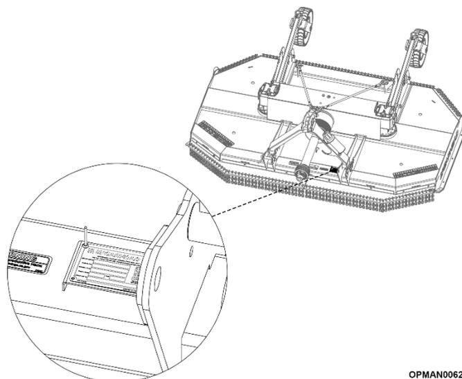
**Figure 1.4 – Serial Plate Location**
