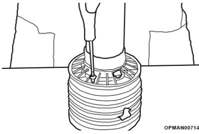
5.3.3.8 Tighten the Phillips head screws. Use of electric powered screwdrivers is not recommended
