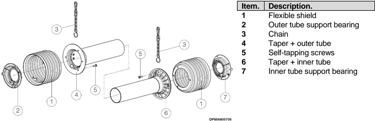
Figure 5.8/Table 5.8 - Input Shaft Safety & Wearing Components
