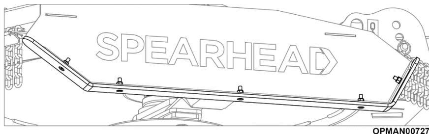
**Figure 5.36 – Multicut Wing Skid**
