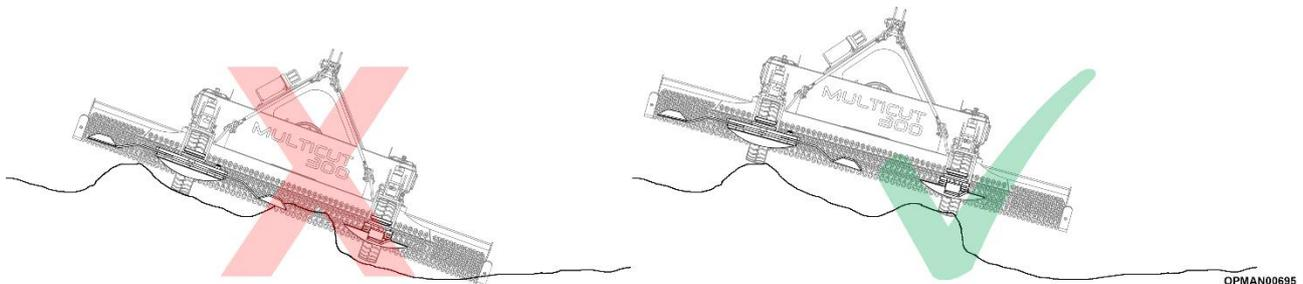
Figure 4.22 – Uneven Ground, Ride On The Tyres Not The Blade Carrier
