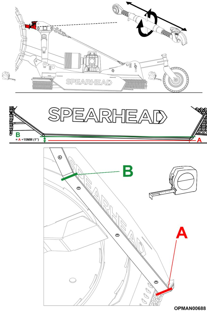
Figure 4.9 – Multicut 300 Front To Rear Machine Levelling
