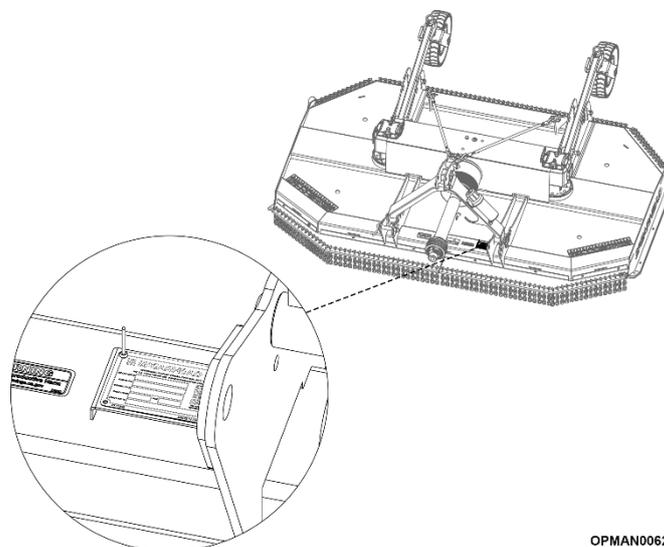
**Figure 1.4 – Serial Plate Location**
