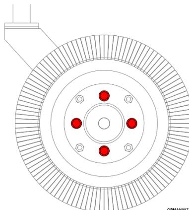
**Figure 5.34 – Multicut Laminated Wheel Nuts To Loosen**
