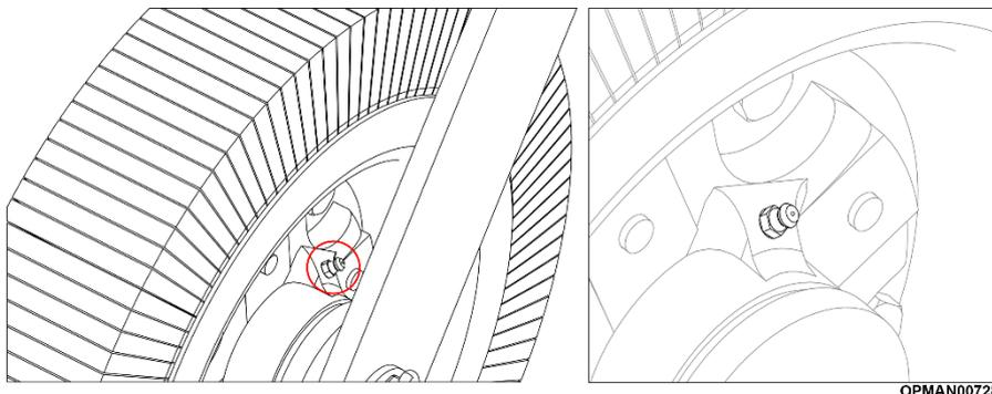
**Figure 5.35 – Multicut Laminated Wheel Hub Greasing Location**
