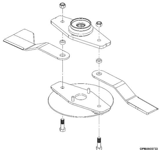
**Figure 5.20 – Multicut Blade Carrier Assembly (standard shown)**
