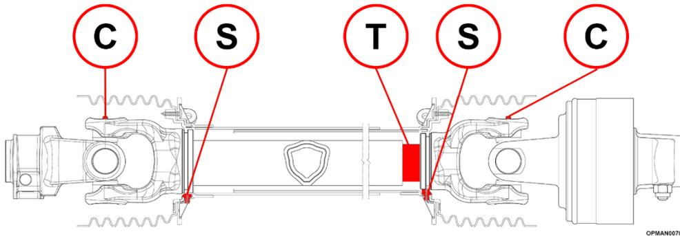
**Figure 5.5 – Multicut Input Shaft Grease Locations**
