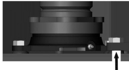
Shim where required to adjust alignment
