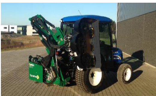
Photo 2: After connecting the RC rotary head to the reach arm the hydraulic hoses can then be attached. Pay close attention to the correct attachment!
