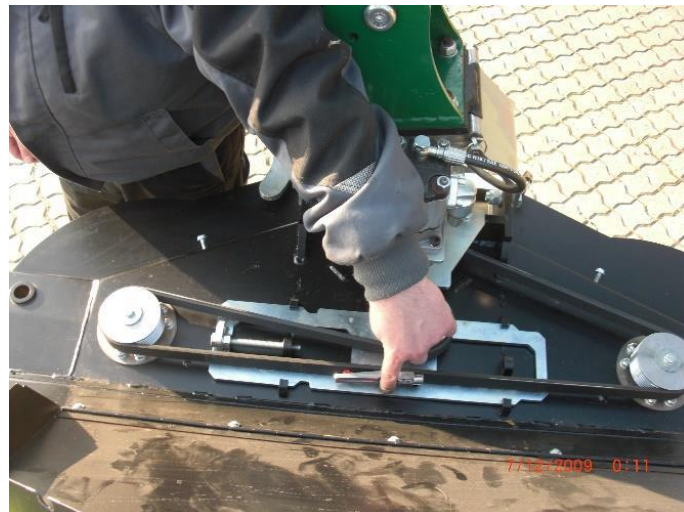
Check belt tension at the middle of the belt with belt measurer 200155.0
