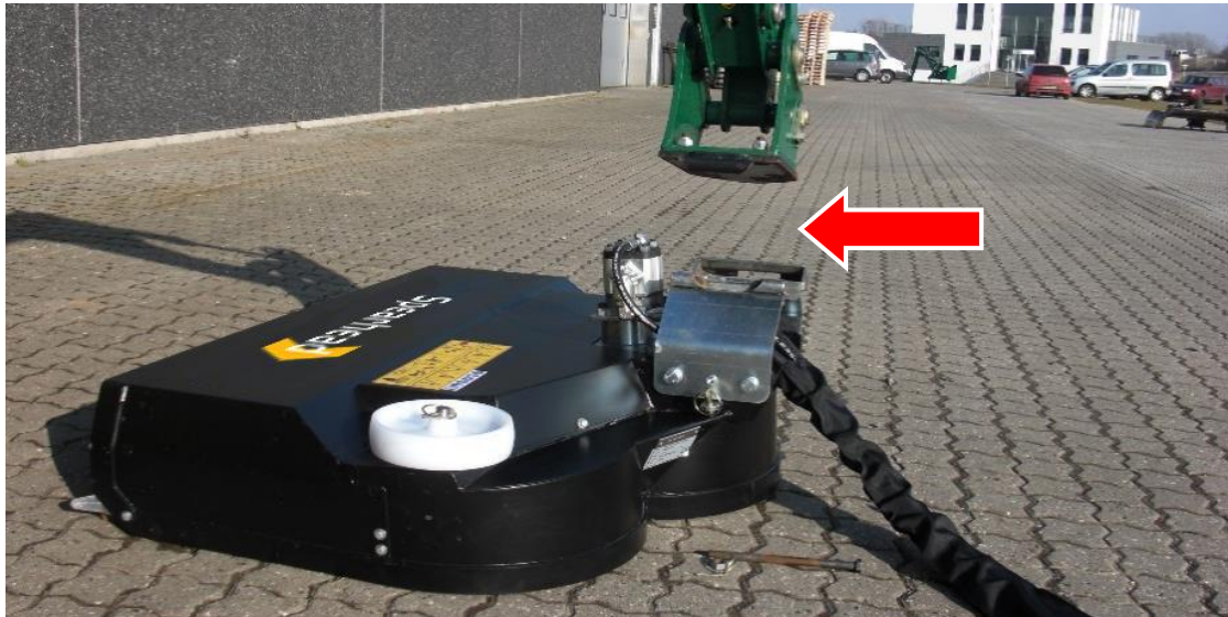
Photo 1: Slowly drive forward and adapt the angle to the RC rotary head. Connect the armsystem and the head.
