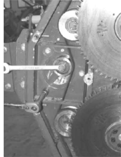
Loosen bolt and turn idler roller
