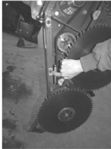
Set tension of lower belt
