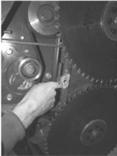
Set tension of the centre belt
