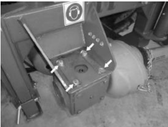
Centre Gearbox Mounting Bolts Location
