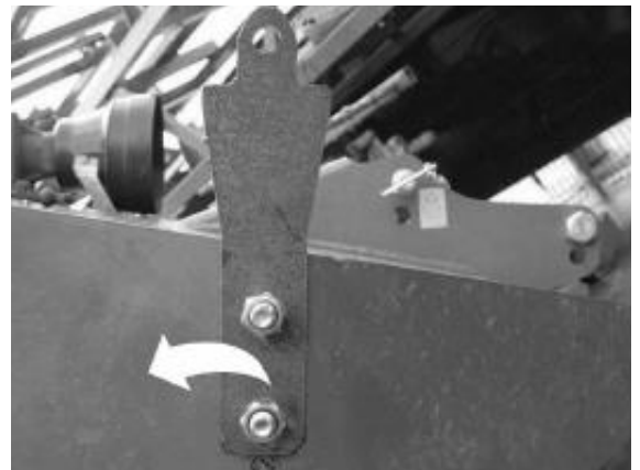
Remove stacking/transport legs (if fitted)
