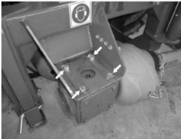
Primary Gearbox Mounting Bolts - Agricut 240 Models only
