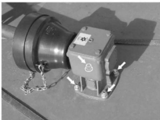
Gearbox mounting nuts and bolts location
