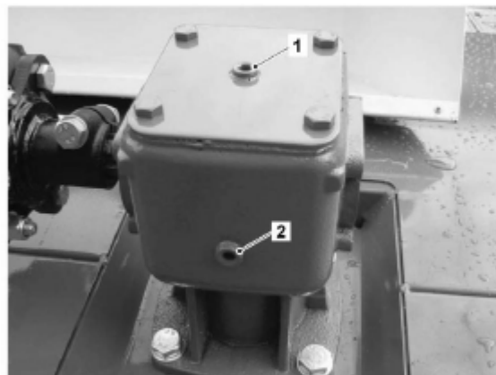
Outer Gearbox Plug Locations (RH shown) 1) Oil Filler Plug 2) Oil Level Plug
