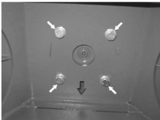
Centre Gearbox Mounting Bolts Location
