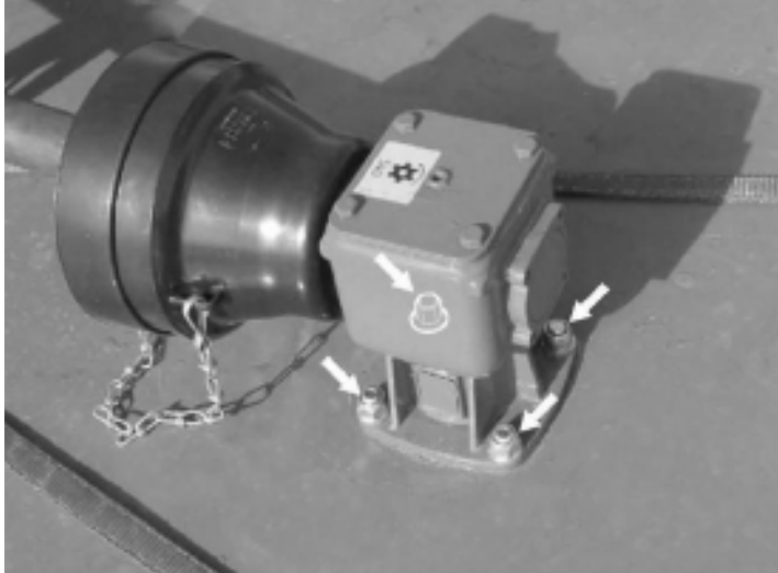
Gearbox mounting nuts and bolts location
