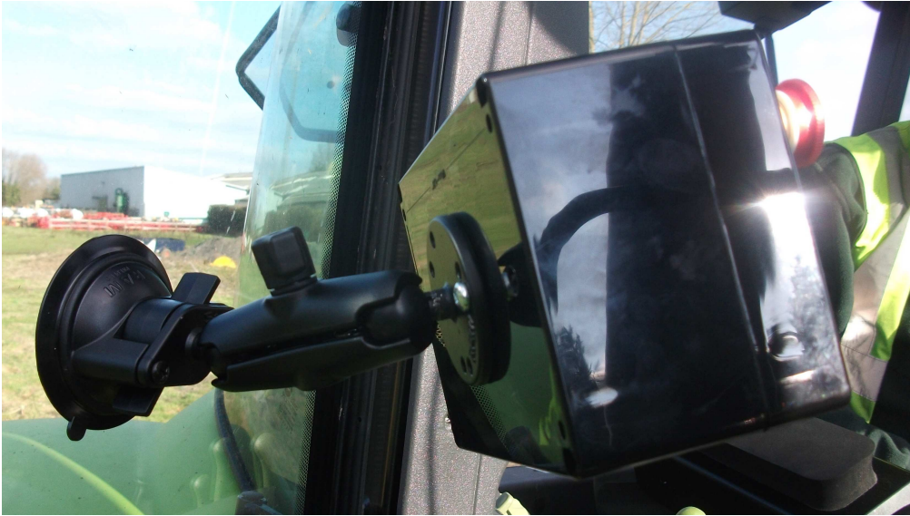
The switch box is supplied with a suction pad to allow the box to be mounted to the tractor cab window for ease of reach.
