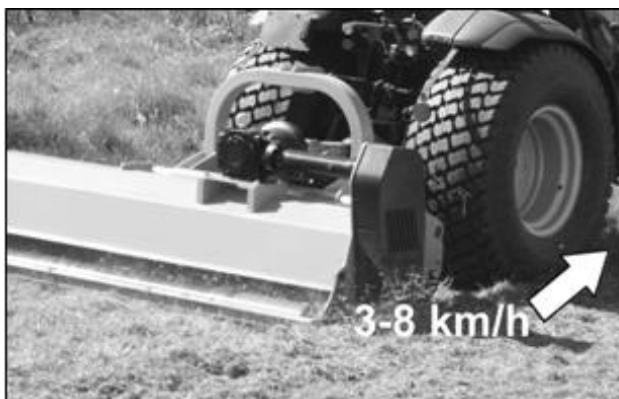
Optimal forward working speed 3-8 km/h
