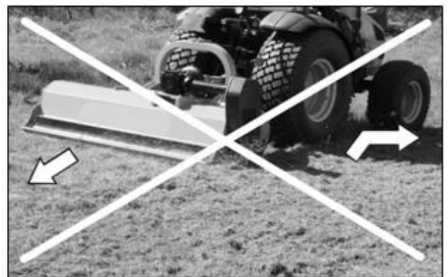
Raise the machine before turning or reversing
