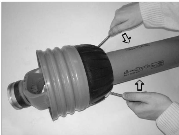
Prise clasps open to release the shield
