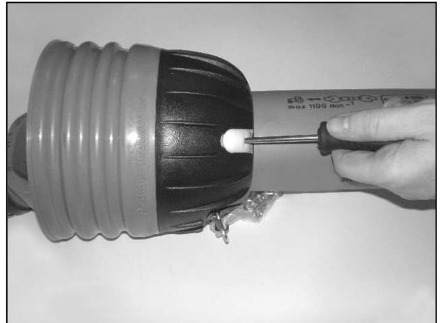
Insert screwdrivers into the clasps
