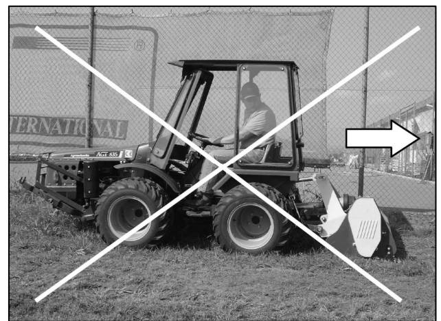
Raise the machine before turning or reversing
