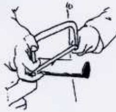
Fig.1 Shortening the PTO drive shaft
